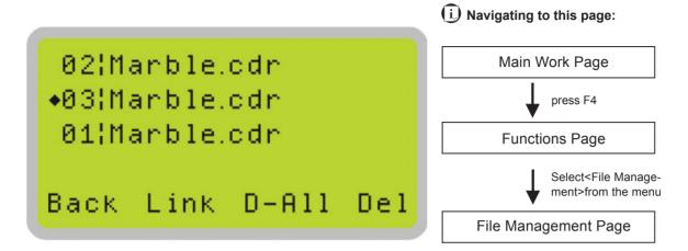
The File Management Page allows you to manage the files that you have loaded onto the LaserPro Spirit GX. You can scroll through your jobs, delete a selected job, delete all jobs, and go to the Link / DLink Page to set and arrange multiple loaded jobs into a single job queue for processing.
