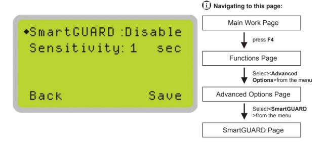
After hardware installation, please enter the function menu on the control panel to enable the SmartGUARD fire alarm.
