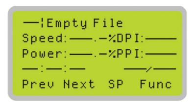
The main work page is the page that the LaserPro Spirit GX will default to upon startup and will be the "home base" for when navigating through the various functions of the control panel. This will be the page that is displayed when you are processing your jobs. This page contains specific job information such as the current job's name, Speed, Power, PPI, DPI, processing / remaining times, and jobs loaded.
