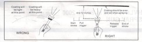
\*TO avoid the over-volume of paint output to get desired pattern, you should better use the lowest pressure.
