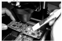
2) Put the tin ball and spread soldering flux (not too thick, only a thin layer of it) on
